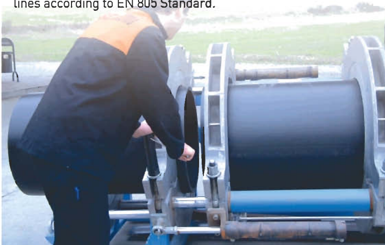
FKS pipe butt welding joint point section.
