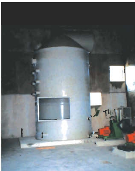
Example of tank produced from PP
