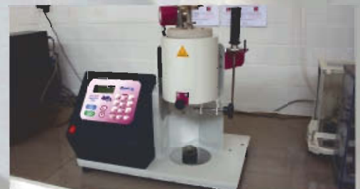
Melt Flow Rate Test
